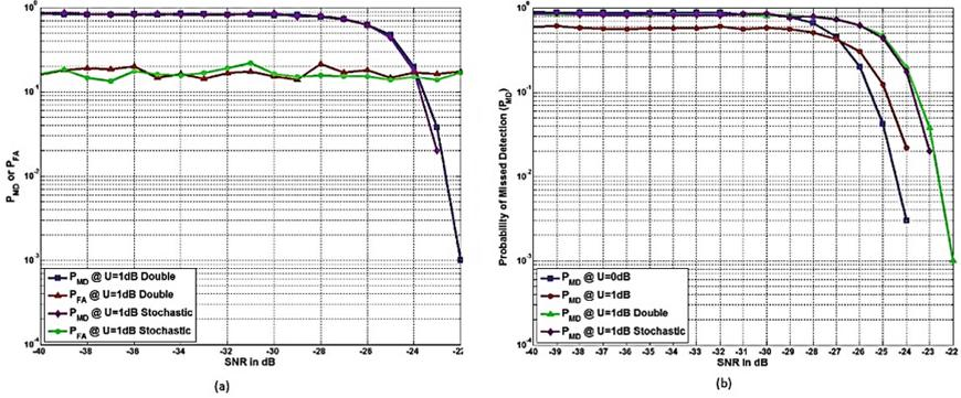
**Fig. 5.** a) For different SNR, probabilities of false alarm and missed detection of the stochastic and double thresholds at  $U = 1$  dB noise uncertainty. b) For different SNR, Missed detection probability for the old threshold at  $U = 0$  dB and  $U = 1$  dB noise uncertainty, and the double and stochastic threshold under  $U = 1$  dB noise uncertainty.
