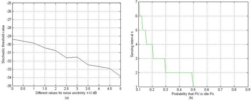
**Fig. 6.** a) Stochastics threshold values for different noise uncertainty. b) The interval of sensing as a function of  $p_i$ .
