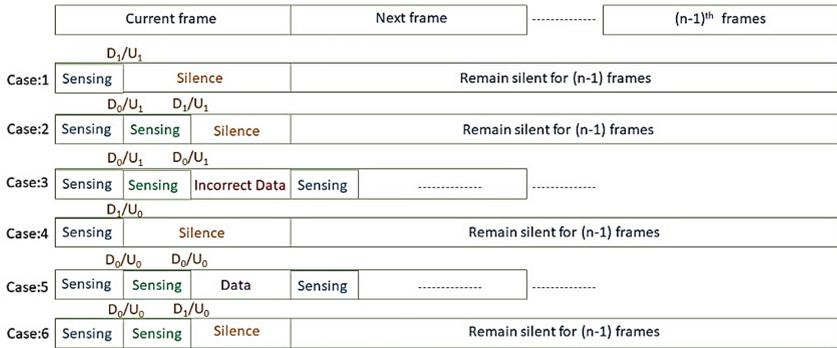
**Fig. 3.** Sensing time and sensing interval frame structure.
