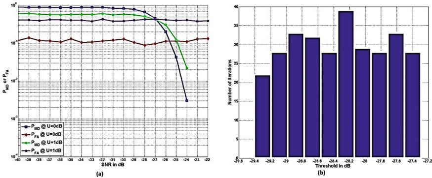
**Fig. 4.** a) For different SNR, missed detection prob. and false alarm prob. of the old threshold at  $U = 0$  dB and  $U = 1$  dB noise uncertainty respectively. b) Histogram for Stochastic-threshold in dB at environment of noise uncertainty.
