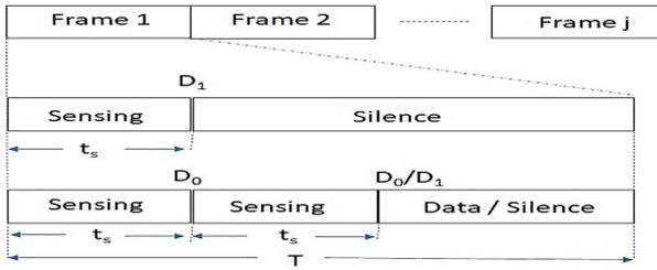
**Fig. 2.** Structure of spectrum sensing frame.
